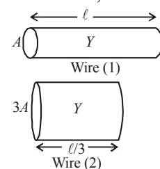
As shown in the figure, the wires will have the same Young's modulus (same material) and the length of the wire of area of cross-section  $3A$  will be  $\ell/3$  (same volume as wire 1).
