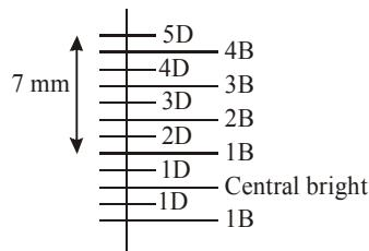
$$\Rightarrow \beta = \frac{7 \text{ mm}}{3.5} = 2 \text{ mm} \Rightarrow \lambda = \frac{\beta D}{d} = 600 \text{ nm}$$
