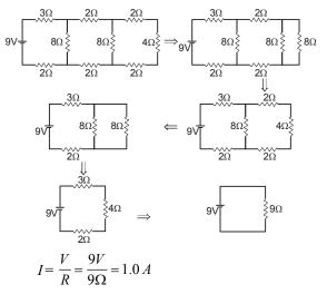
The flow of current in the circuit is as follows.
