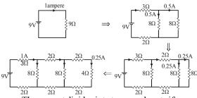
The current divides into two equal parts if passes through two equal resistances in parallel. Thus current through  $4\Omega$  resistor is 0.25 A.
