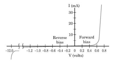
Estimate the dynamic resistance of diode at V = -0.6 volt.
