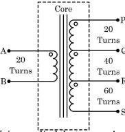
Input voltage of 20 V is applied between A and B. Between which two terminals will the output be 120 V?
