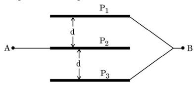
(i) The capacitance of the system between A and B will be:
