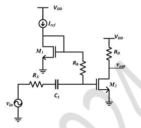
Assuming that capacitor  $C_1$  is a short circuit for AC analysis, the exact magnitude of small signal voltage gain  $\left|\frac{v_{out}}{v_{in}}\right|$  is \_\_\_\_\_.
