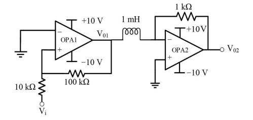
Assume that the initial inductor current is 0 A. The input voltage (V<sub>i</sub>) is a triangular signal with peak voltages of  $\pm 2$  V and time period of 8 µs. Which one of the following statements is true?
