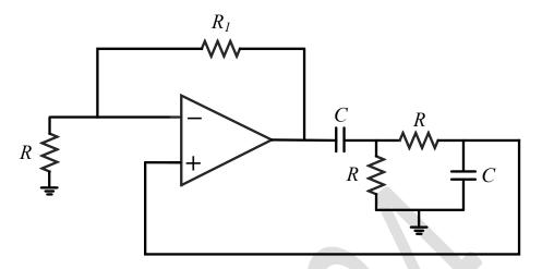
If the circuit is to show sustained oscillations, the respective values of  $R_1$  and the corresponding frequency of oscillation are \_\_\_\_\_.
