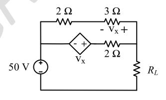
The value of  $R_L$  (in  $\Omega$ ) is \_\_\_\_\_.
