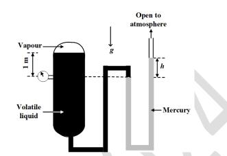
The height, h (in m, rounded off to two decimal places) of the mercury column in figure is \_\_\_\_\_.
