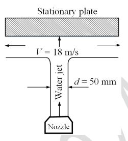
The magnitude of net force (in N, *rounded off to two decimal places*) imparted by the jet on the stationary plate is \_\_\_\_\_\_.
