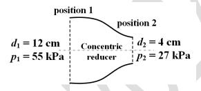
Neglecting frictional effects, the mass flow rate (in kg/s, *rounded off to two decimal places*) of the fluid through the reducer is \_\_\_\_\_.
