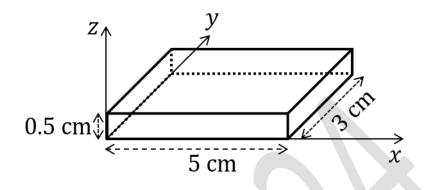
When the majority charge carrier concentration is  $12.5 \times 10^{13}$  cm<sup>-3</sup> and the sample is exposed to a constant magnetic field applied along the +z direction, a Hall voltage of 20 mV is measured with the negative polarity at y = 0 plane. Take the electric charge as  $1.6 \times 10^{-19}$  C. The concentration of minority charge carrier is negligible. Which of the following statement is/are true?
