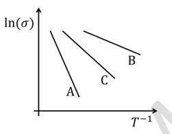
Let  $E_A$ ,  $E_B$  and  $E_C$  be the bandgaps of A, B and C, respectively. Which one of the following relations is correct?
