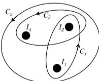
If the value of the integral  $\oint_C \vec{B} \cdot \vec{dl}$  for the loops  $C_1$ ,  $C_2$ , and  $C_3$  are  $2\mu_0$ ,  $4\mu_0$ , and  $\mu_0$  in the units of N/A, respectively, then
