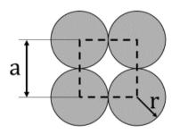
The percentage (%) area occupied by the grey circles (of radius r) inside the unit cell is \_\_\_\_\_. (*rounded off to the nearest integer*)
