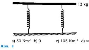
Sol.  $T = 2\pi \sqrt{\frac{m}{k_{eff}}}$  $\frac{3}{2} = 2\pi \sqrt{\frac{12}{2k}}$  $\frac{9}{4} = 4\pi^2 \times \frac{12}{2k}$  $k \simeq 105 \text{ n/m}$
