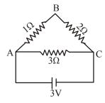
Here, two reisistance of  $1\Omega$  and  $2\Omega$  are in series, which form  $3\Omega$  which is in parallel with  $3\Omega$  resistance.
