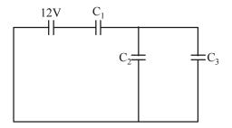
Now,  $C_{eq}$  and  $C_1$  are in series. Therefore, their equivalent capacitance is
