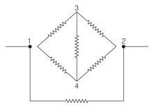
It is circuit of Wheatstone the equivalent resistance of upper circuit
