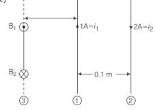
According to question, the third wire should not feel magnetic force due to wire (1) and (2). It can be only possible in the condition
