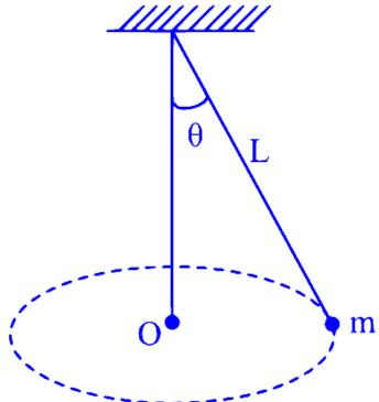
A small ball of mass m is suspended from the ceiling of a floor by a string of length L. The ball moves along a horizontal circle with constant angular velocity  $\omega$ , as shown in the figure. The torque about the centre (O) of the horizontal circle is
