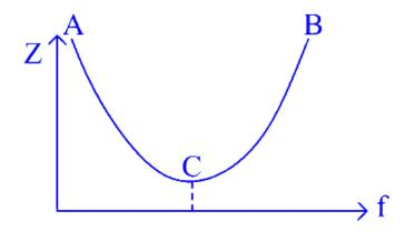
The variation of impedance Z of a series LCR circuit with frequency of the source is shown in the figure. Which of the following statement(s) is/are true?
