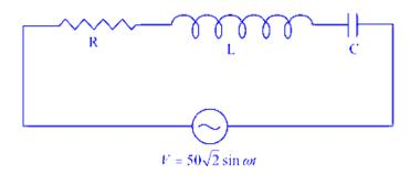
In a series LCR circuit, the rms voltage across the resistor and the capacitor are  $30~\rm V$  and  $90~\rm V$  respectively. If the applied voltage is  $50\sqrt{2}\sin\omega t$ , then the peak voltage across the inductor is
